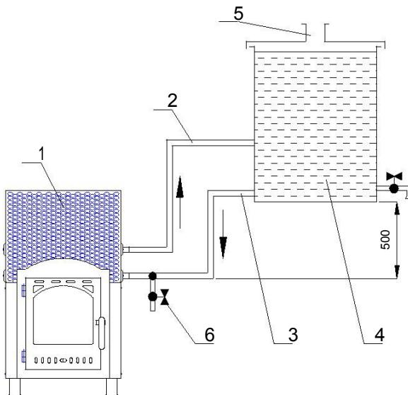
**Chart for the connection of the sauna heater:** 1. Heater. 2. Hot water pipe. 3. Cold water pipe. 4. An open tank of water. 5. Branch (opening). 6. Water release valve.
